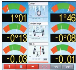
Front meter screen with frozen readings - freezes the readings to allow the technician to lift or move the vehicle then make the readings live again.
