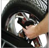
Accu-stik parameter entry arm holds the weight while the screen shows the technician where to place it
