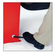
Standard foot brake locks the shaft to eliminate accidental tire roll while applying weights
