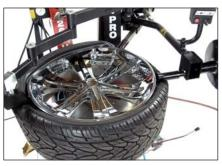
Accu-Pro Mounting Helper shown easily mounting the top bead on 26" rim.
