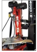
Unique telescoping tower allows for wide rims and produces added strength.
